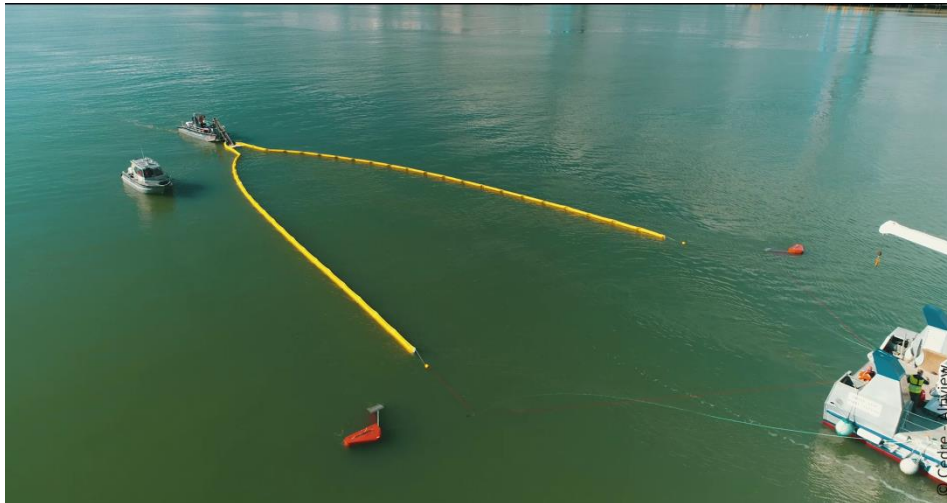
Photo 31 : Trials on the Loire of the R3S (V-shaped boom and skimmer on a support boat) connected at the apex of the booms. The system is towed by a single boat assisted by two paravanes (Source: Cedre – Altiview)
