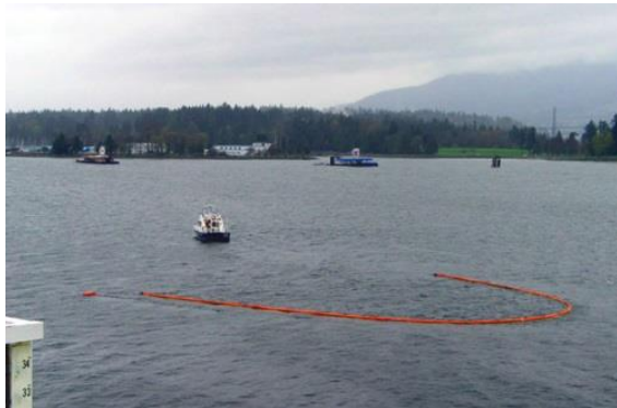
Photo 1: Boom and Trawl boom towed by one vessel equipped with a paravane (source Cedre)
