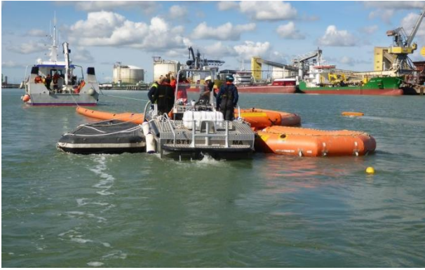
Photo 14 : The support boat and Aristock alongside the CB2 in preparation for pumping while towing continues at reduce speed (source: Cedre)
