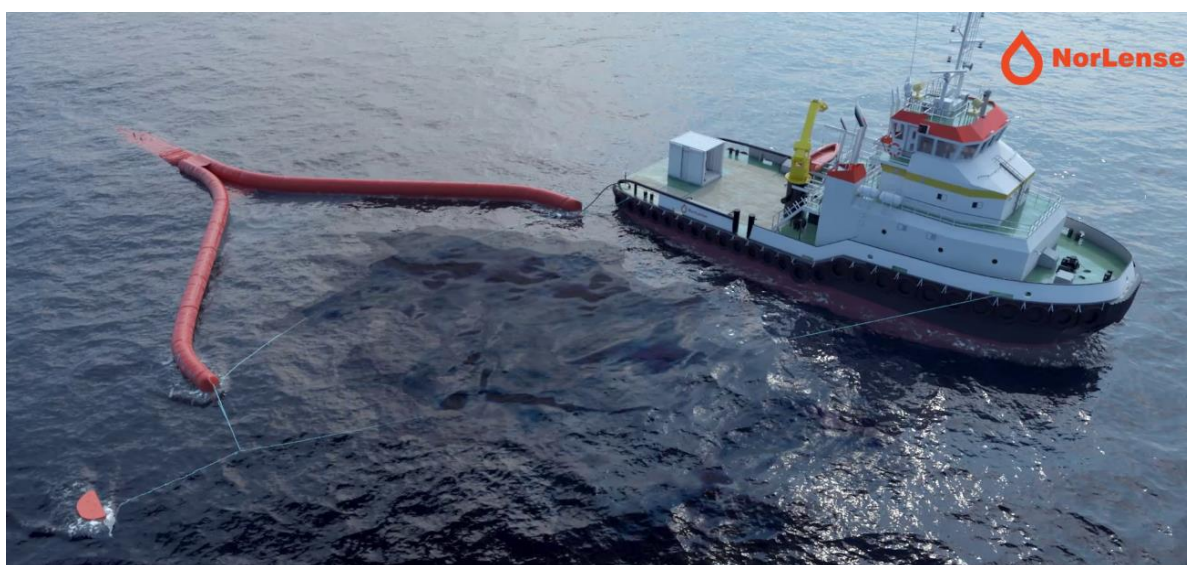
Photo 36 : Overall view of the Oil Trawl system towed by a single vessel using the Trawldoor paravane, (source: NorLense)
