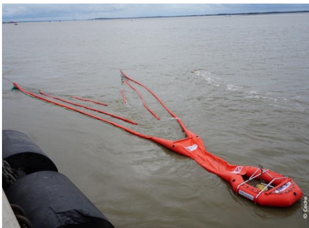
Photo 23 : Deflector booms, tunnel and pool (source: Cedre)
