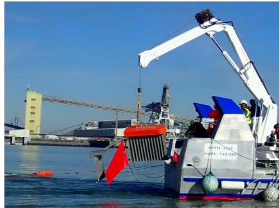
Photo 35 : Deploying the BoomVane™ using the crane onboard the towing vessel (source Cedre)
