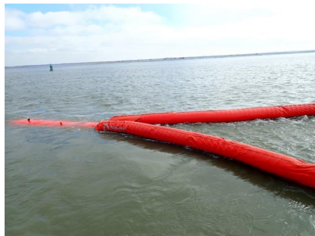
Photo 38 : Close-up of the apex of the system and the floating bag (Source Cedre)
