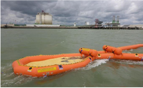
Photo 17 : Waves coming from behind, surface speed of 3.6 knots, satisfactory containment (source: Cedre)
