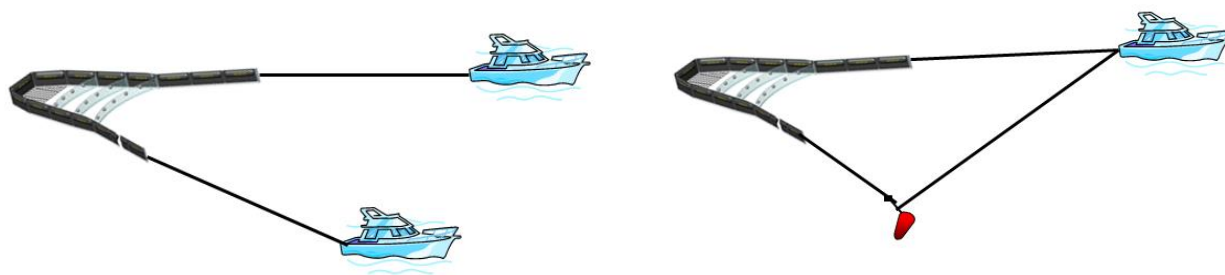
Fig. 18 – Schematic diagram of the device towed by 2 boats and by a single boat with a paravane (source: Cedre)
