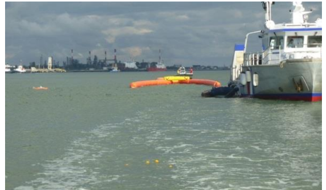
Photo 2: Examples of dynamical booming configurations (source: Cedre)
