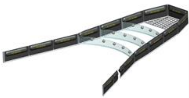
Fig.17 – Diagram of the Desmi Speed Sweep (source: DESMI).
