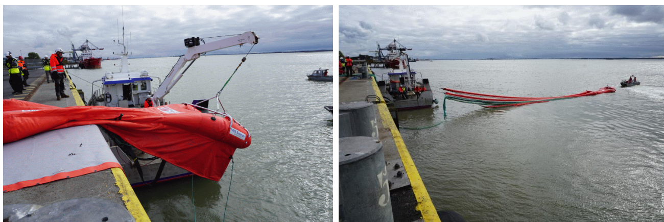
Photo 29, Photo 30: Deployment of LMOS 15 from a dock using the hydraulic crane of the work vessel provided by the Lighthouses and Beacons subdivision of Saint-Nazaire (Source: Cedre)
