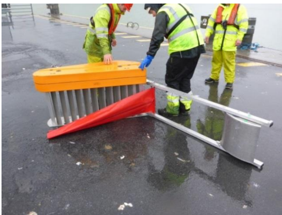
Photo 11, Photo 12 : View of the BoomVane on the dockside prior to deployment and on the water (Source: Cedre).
