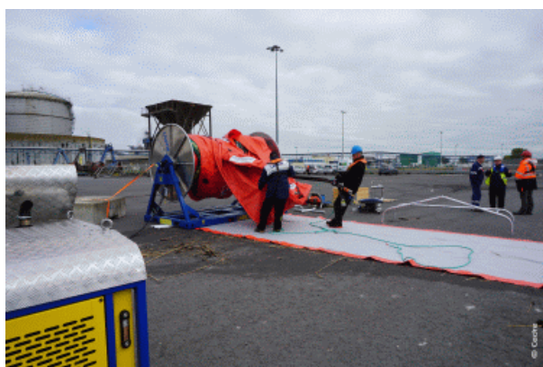
Photo 27, Photo 28 : Deployment using a boom reel on a dock in Saint-Nazaire (Source: Cedre)
