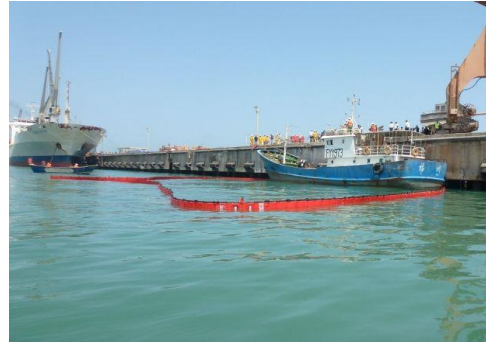
Photo 5, Photo 6 : Containing oil against a structure (source Cedre)
