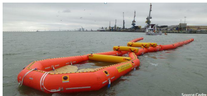
Photo 16 : View of the current buster 2 towed by a vessel an Boom Vane paravane (source: Cedre)
