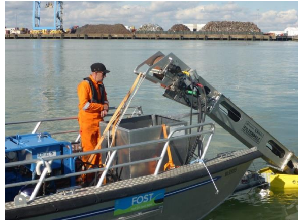
Photo 33 : The Marco FilterBelt Skimmer in operation (source Cedre).
