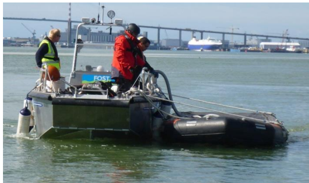
Photo 13 : An Aristock floating storage tank alongside the the operating support boat (source: Cedre).
