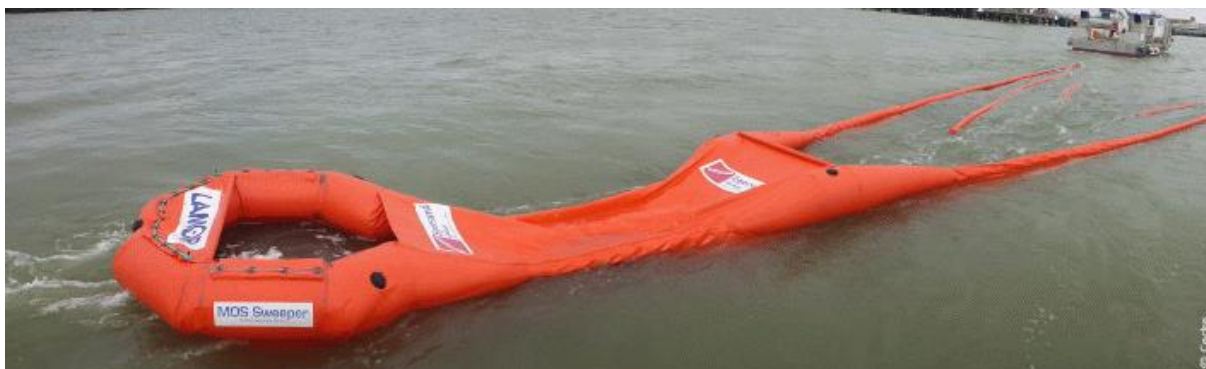
Photo 25 : Detail of the tunnel and the pool of the LMOS 15 (source: Cedre)
