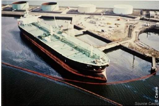
Photo 5, Photo 6 : Containing oil against a structure (source Cedre)
