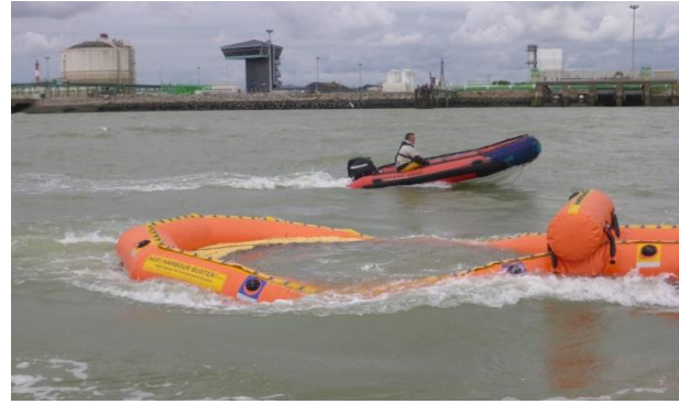
Photo 18 : Waves coming from behind, surface speed of 4.1 knots, leakage (source: Cedre)
