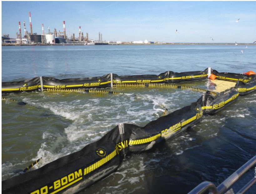
Photo 21 : Surface current attenuation within the Speed Sweep during test in the Loire estuary (Source: Cedre)
