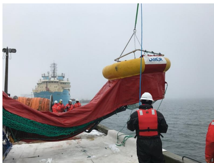
Photo 26 : Bottom net visible during the deployment (Source: Lamor)
