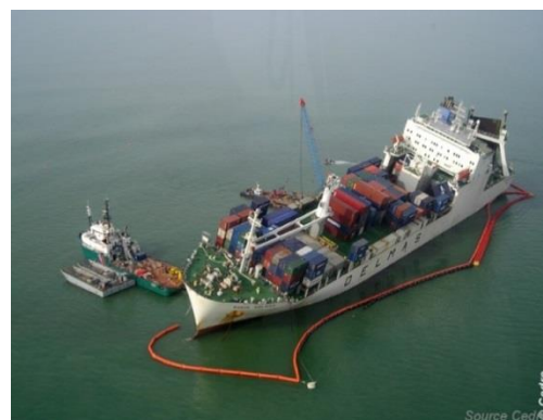
Photo 3, Photo 4 : Corraling a vessel (source Cedre)
