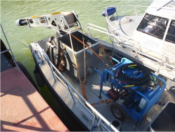
Photo 32 : Overview of the on-board set-up: hydraulic power pack, mounting tank and Marco FilterBelt Skimmer (source Cedre).
