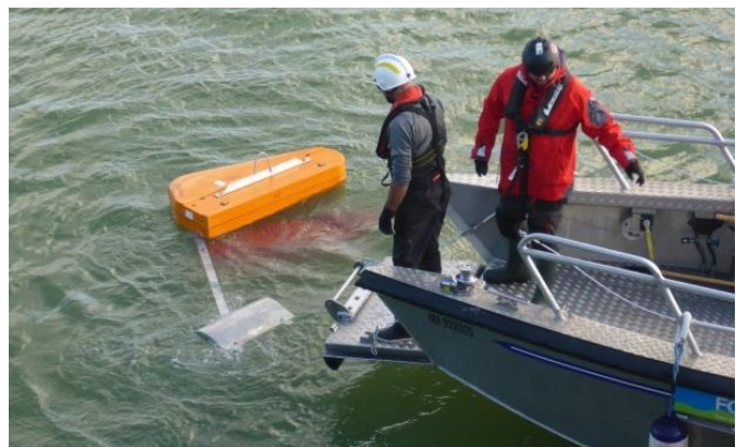
Photo 11, Photo 12 : View of the BoomVane on the dockside prior to deployment and on the water (Source: Cedre).
