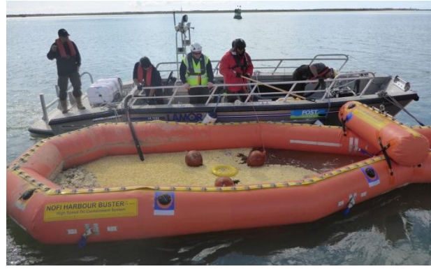
Photo 15 : Recovering the simulated spill (popcorn) by using a skimmer in the settling storage pool of the Current Buster 2 for transfer to the floating Aristock tank. (source: Cedre)
