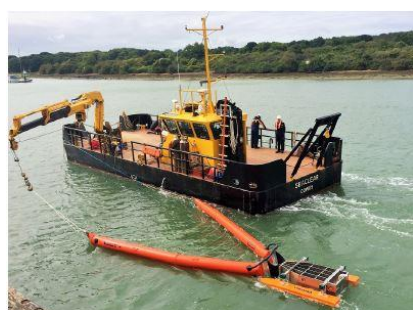
Photo 41 : Fasflo use in dynamic mode as a sweep system alongside an oil response vessel (Source: Vikoma)
