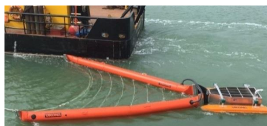
Photo 40 : View of the cross lines between the two booms (source: Vikoma)
